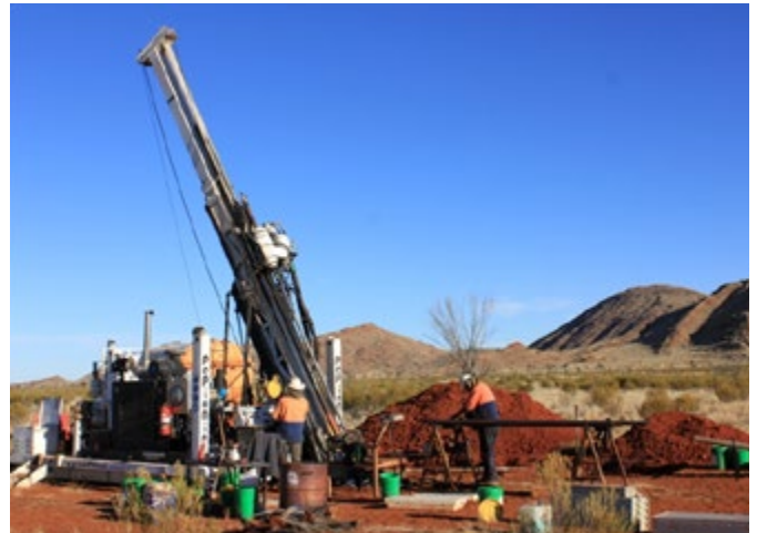
Figure 2: PepinNini Diamond Core Drilling Rig
