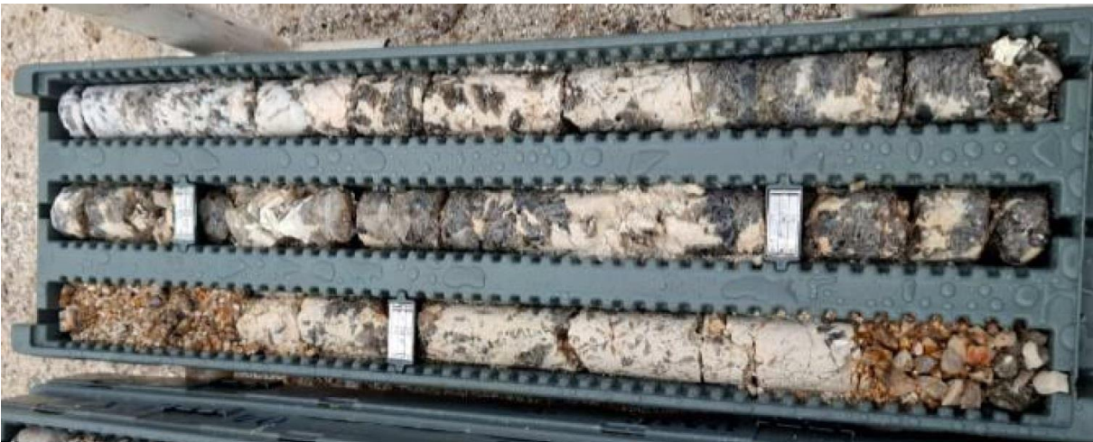
Figure 1: Drill core from hole PMB25-04, showing a section from 14m-17m depth
