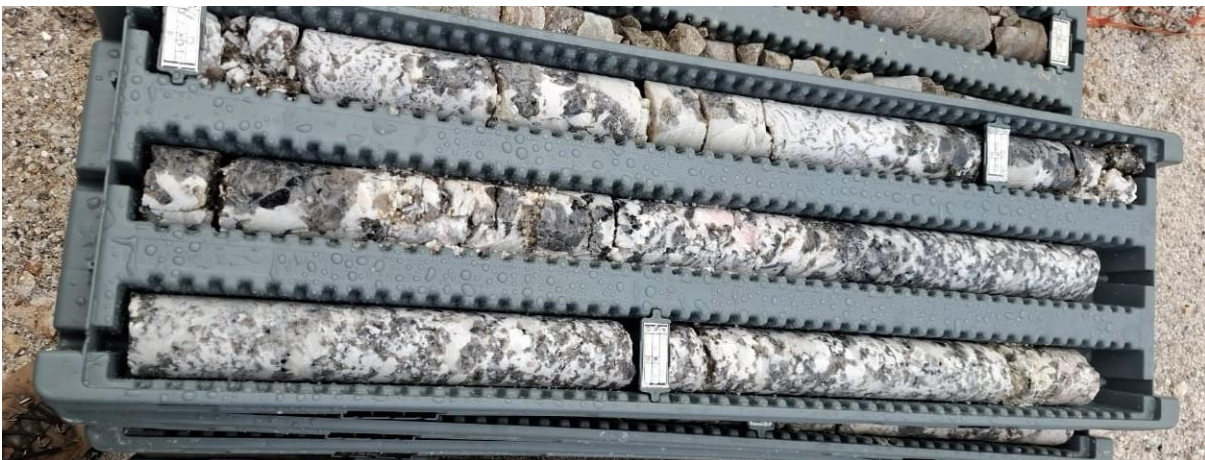
Figure 2: Drill core from hole PMB25-04, showing pegmatite a section 3.3 to 6.2 metres down hole.
