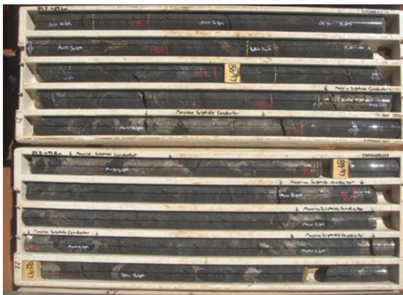
Figure 4 – DD13WOD017 from depth 84 to 93 metres: image showing massive to semi-massive pyrrhotite hosted within a sulphidic pyroxenite and gabbronorite.
