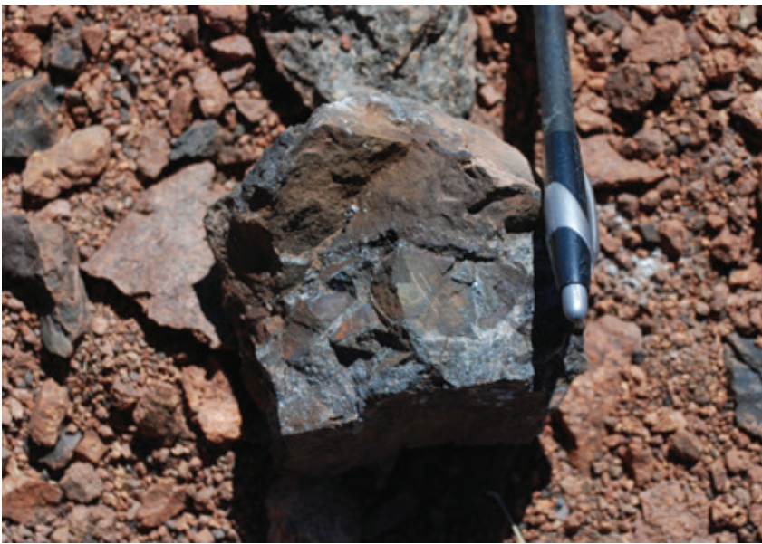
Figure 12 – Haematite matrix breccias with trace copper mineralisation from within major shear zone located near the ‘El Obsequio’ epithermal Cu-Au prospect.
