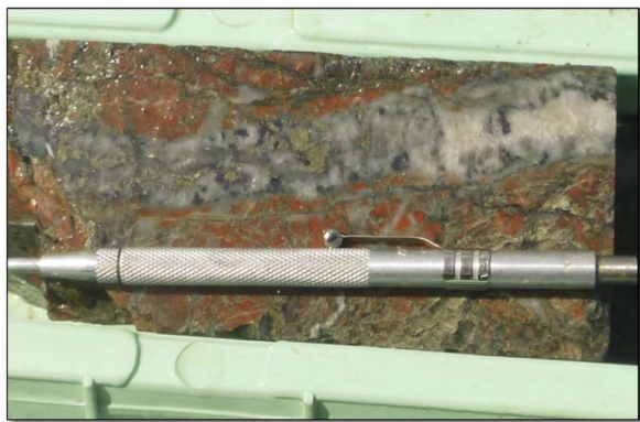
Photo 2 Quartz Carbonate vein at Minos with an interval of 1m at 10 grams per tonne Gold
