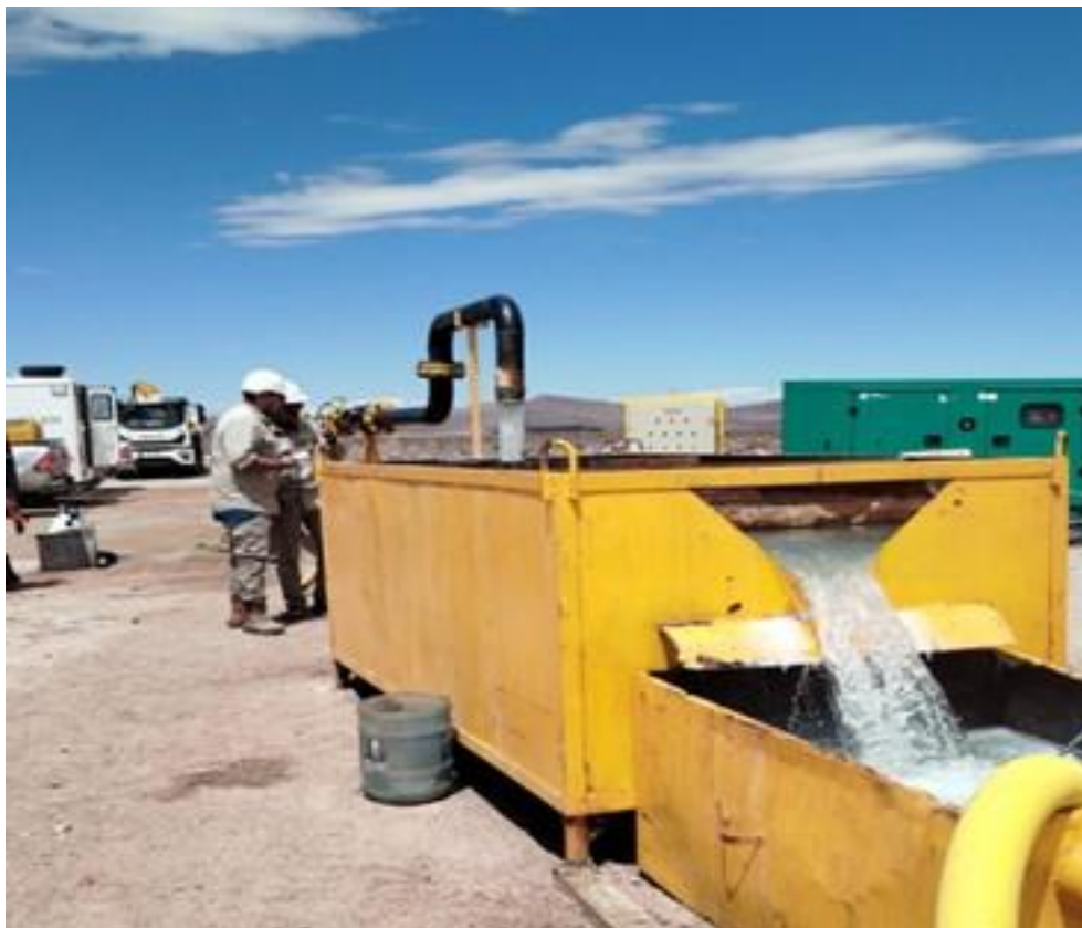
Figure 4: Pumping well tests in progress at Incahuasi Project.
